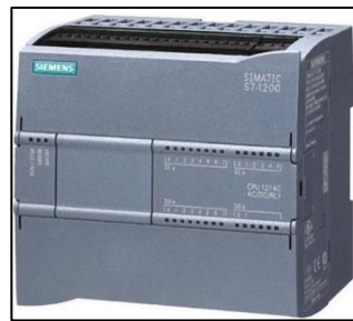
Figura 12. PLC SIMATIC S7-1200.
