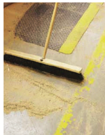
Sawdust is dry contamination that can create a slip hazard.
