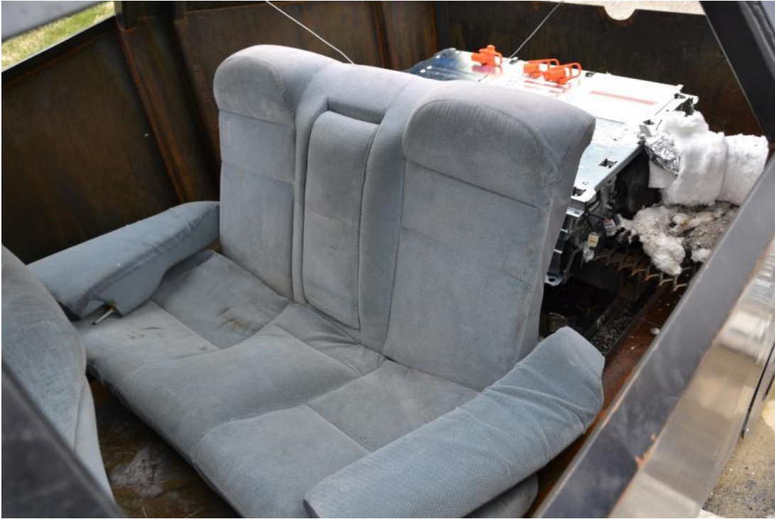
Figure 32 Back seats installed inside the VFT for Test A3
