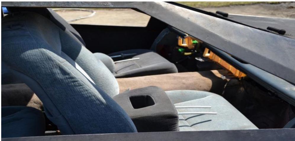
Figure 37 Dashboard, front seats, and carpet installed inside the VFT for Test B3
