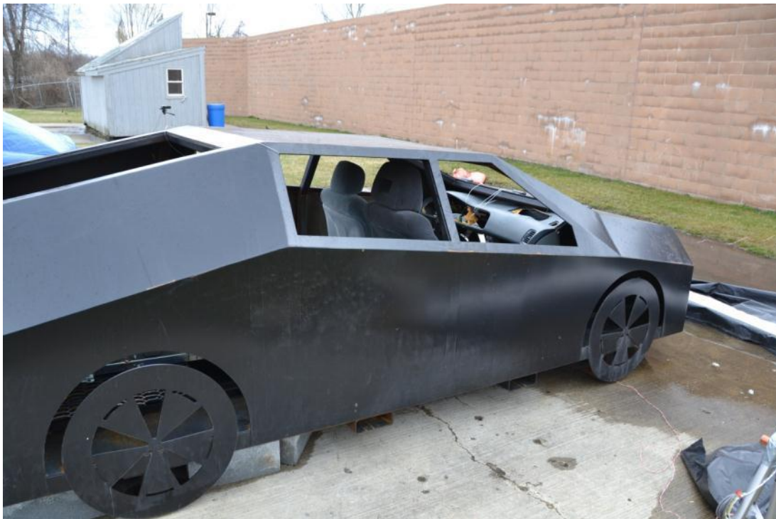
Figure 29 Overall view of the VFT with interior finishes for Test A3
