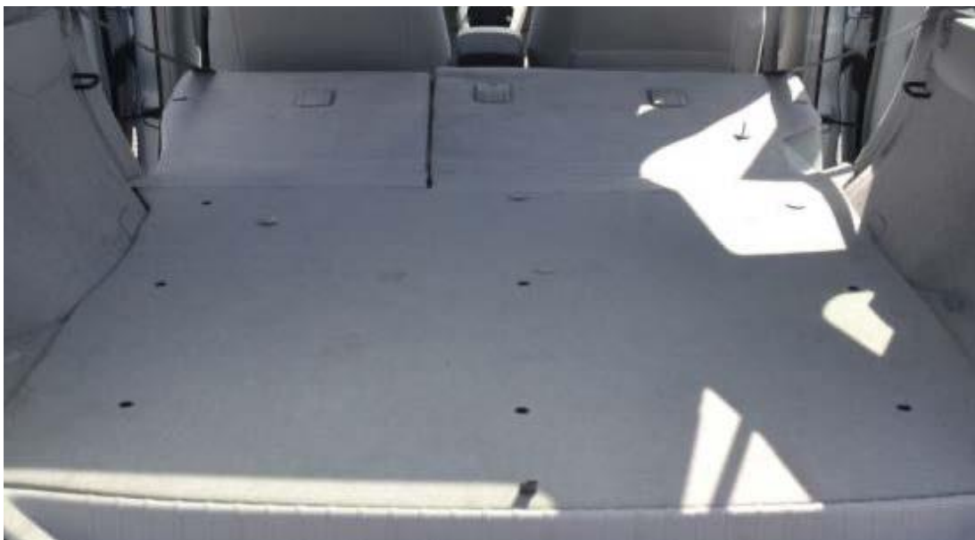
Figure 7 Battery A cargo area over the battery compartment
