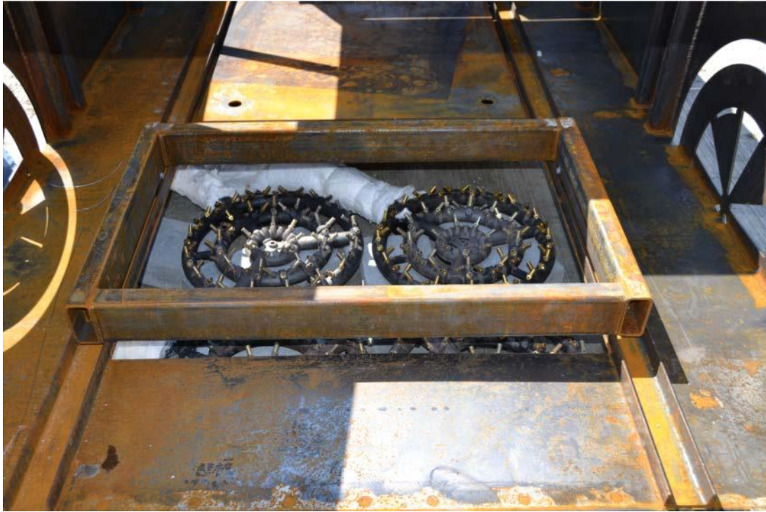
Figure 25 Carriage installed inside the VFT positioned above the four burners located in the rear test position
