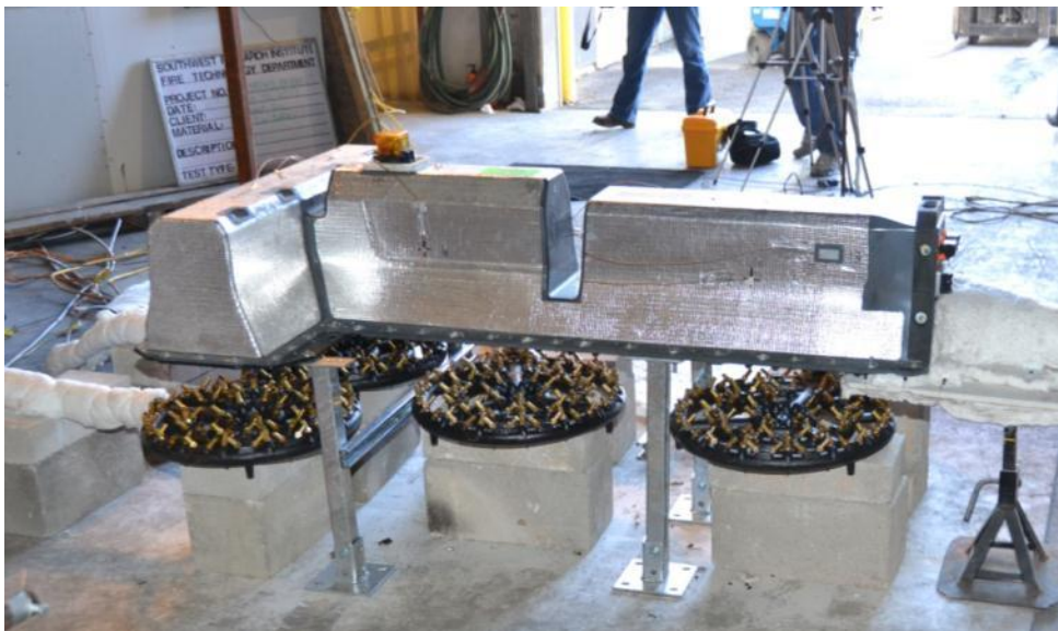
Figure 16 Four burners positioned under Battery B
