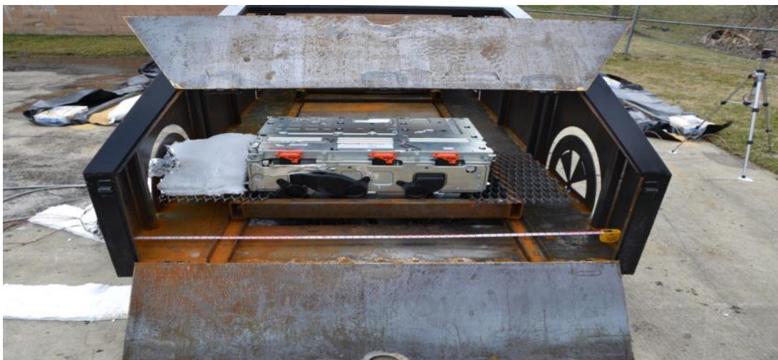
Figure 26 Battery A positioned on the carriage above the burners and inside the VFT
