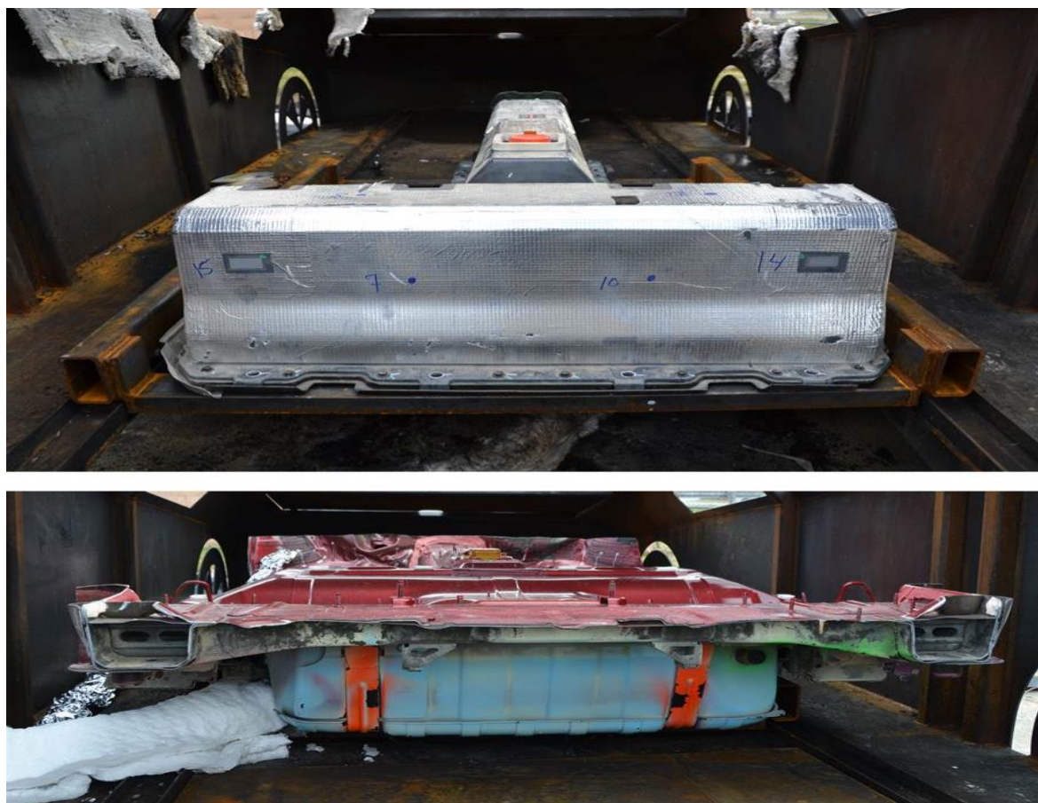
Figure 34 View of Battery B inside the VFT without the floor pan (top) and with the floor pan (bottom); the blue tank at the rear of the battery is the empty gasoline tank for the production vehicle, which blocks direct access to the rear of the battery
