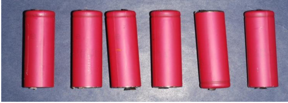
Figure 3 Example of 18650 cylindrical cells (these are the most common consumer electronics Li-ion cell form factor)
