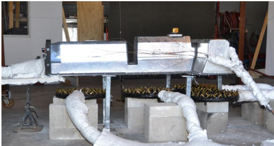
Figure 11 Battery B configuration and burner locations for HRR testing
