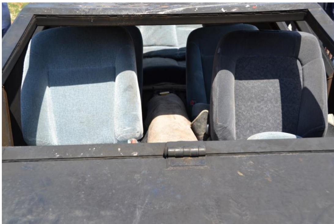
Figure 38 Front seats and carpet installed inside the VFT for Test B3
