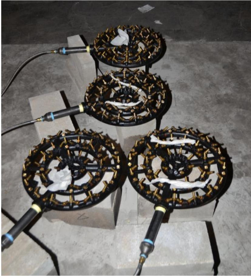
Figure 15 T-shaped burner arrangement comprised of four burners
