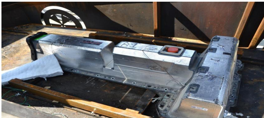
Figure 27 Battery B positioned on the carriage above the burners inside the VFT; burners located in the center test position
