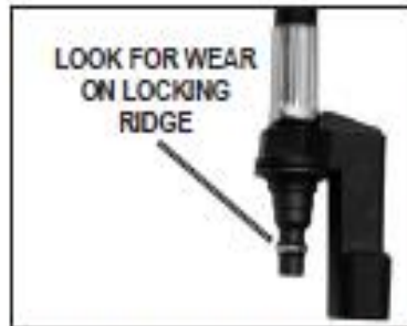
FIGURE 6 Inspecting Male Quick Disconnect
