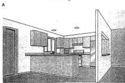
Figure 5-11 A. A load-bearing wall provides structural support. B. A non-load-bearing wall supports only its own weight.
